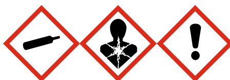
Gas cylinder Health hazard Exclamation mark
